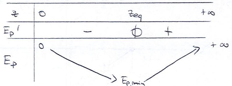
$$E_p(z_{eq}) = -mg(l_0 + mg/k) + \frac{1}{2}k\left(\frac{mg}{k}\right)^2 \\ = -mgl_0 - \frac{1}{2}\frac{(mg)^2}{k} = E_{p,min} < 0$$
