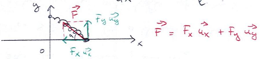
$$F_x = \dots : \| \vec{F} \| \cos(\alpha) \quad \text{et} \quad \cos(\alpha) = \frac{x}{l}$$
