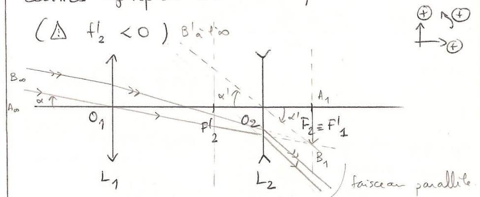
$$\overline{O_1 O_2} = \overline{O_1 F'_1} + \overline{F'_1 O_2} = \overline{O_1 F'_1} + \overline{F_2 O_2} = f'_1 - f_2$$
