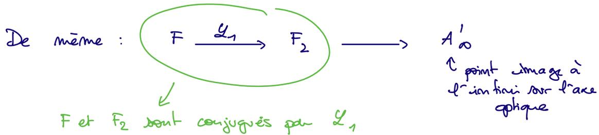
Ainsi  $\overline{F_1 F} \times \overline{F'_1 F_2} = -(f'_1)^2$  donc  $\overline{F_1 F} = -\frac{(f'_1)^2}{\overline{F'_1 F_2}}$
