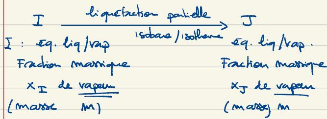
1<sup>er</sup> principe :  $Q_F = \underbrace{m(x_I - x_J) \Delta h_{\text{liq}, T_F}}_{\text{masse de vapeur}} = -m(x_I - x_J) \Delta h_{\text{vap}, T_F}$
